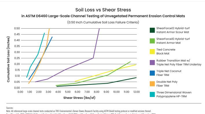
GrassWorx, LLC., 2018. ASTM D6460 Channel Testing of InstaTurf ShearForce 10 EC TRM and ShearForce12 Scour Control Mats in 20% Test Flumes, August, October and December, 2018.
